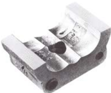
Figure 3: A typical pitting on the pump casing
